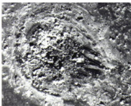
Figure 5. Corrosion in A53 steel. 40 X.
